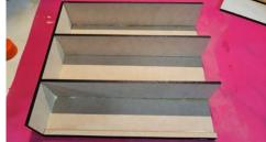
Step 13: Glue the left side piece in place, and attach rubber bands to hold together while drying.
